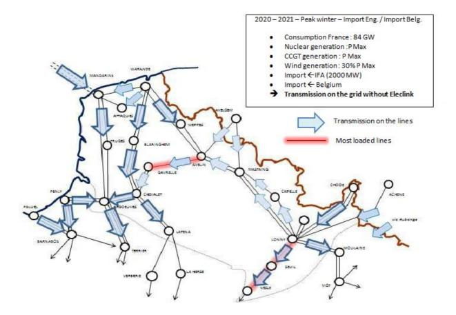
In this situation, which is identical to the previous situation as regards consumption and generation conditions, imports from Belgium amount to around 1 GW (physical flows on the interconnection links) and imports from England amount to 2 GW.
