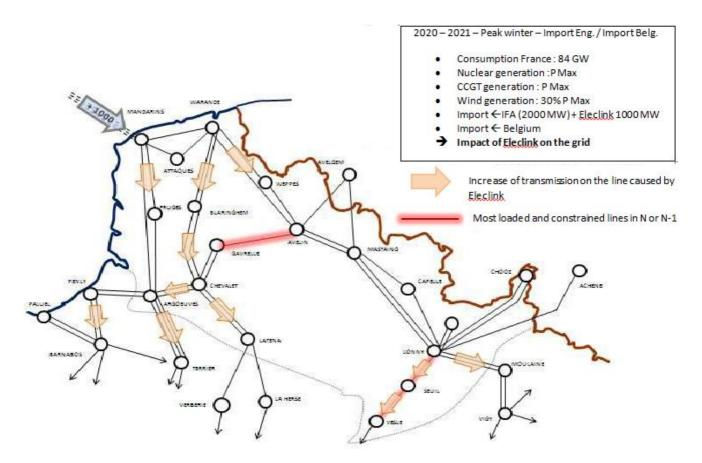
It is noted that Eleclink has a real impact on the 400-kV lines, which are already significantly loaded. Therefore, the additional import of 1000 MW also increases flows on the Lonny-Vesle-Seuil 400-kV line.
