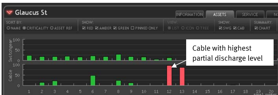
Figure 12 Remote identification of discharging cables
