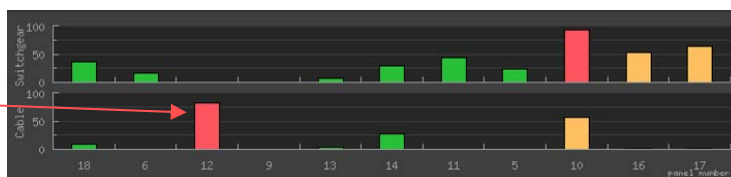
Figure 3 Summary graph highlighting discharging feeders
