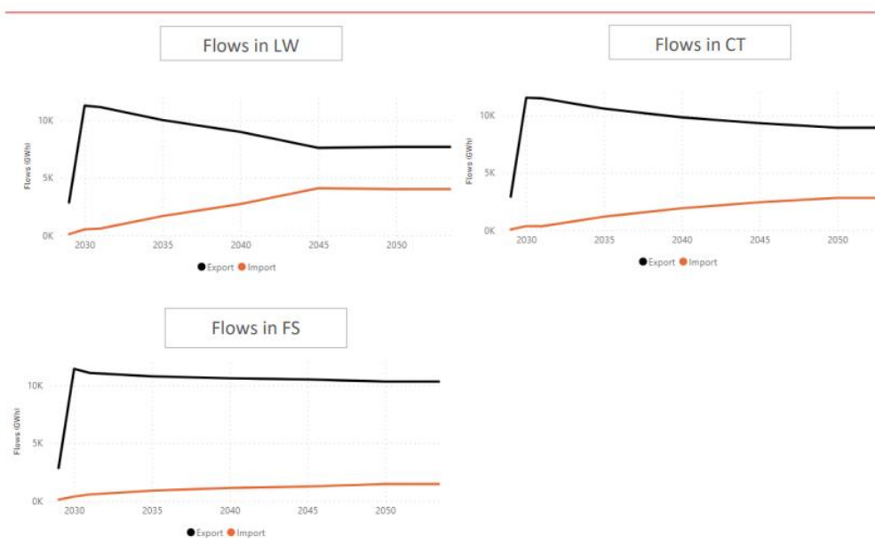
Figure 29 – Electricity flows across Cronos (black line: exports from GB, orange line: imports from Belgium) (GWh)
