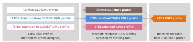
The final LTDS RDFS profiles are included, along with the CGMES v3.0 RDFS profile and the two difference RDFS profiles, in *Appendix 6 – LTDS Profiles in RDFS*.
