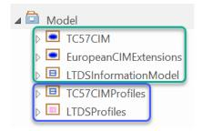
The top three packages (boxed in green) comprise the information model, the lower 2 packages make up the profiles. The TC57CIM package contains the underlying CIM information model, the EuropeanCIMExtensions package contains European and Network Codes extensions and the LTDSInformationModel package contains the Great Britain extensions defined for LTDS.
