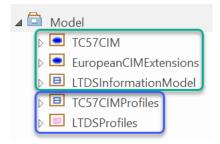
The top three packages (boxed in green) comprise the information model, the lower 2 packages make up the profiles. The TC57CIM package contains the underlying CIM information model, the EuropeanCIMExtensions package contains European and Network Codes extensions and the LTDSInformationModel package contains the Great Britain extensions defined for LTDS.
