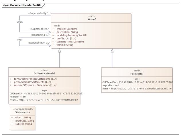
The Model class defines the header information and the md:FullModel and dm:DifferenceModel objects used in exchanges inherit the Model attributes and associations. For LTDS it is defined that all the md:Model attributes, except .version, are required in both the md:FullModel and dm:DifferenceModel objects of LTDS data exchanges. The .version is attribute is considered optional. The md:Model.Supersedes association is not used by LTDS and the md:Model.DependentOn association is conditional.
