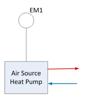
NOTE: The pipes may diverge after they exit the ASHP to feed one (or multiple) space heating loops or a combination of space heating and domestic hot water heating loops. A minimum of one electricity meter is required to measure the input electricity required to run the heat pump compressor and any other electrical input (e.g., for hot water boosting, evaporator fans etc) that has gone into the generated heat output. Potentially more than one electricity meter may be required.
