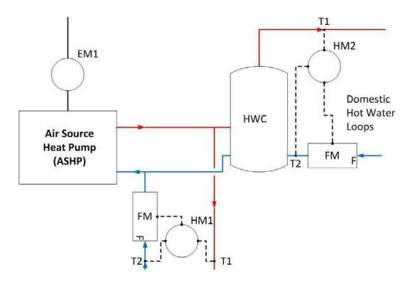
NOTE: One heat meter cannot be installed at the point that the pipes exit the ASHP due to physical constraints therefore must be installed as shown.
