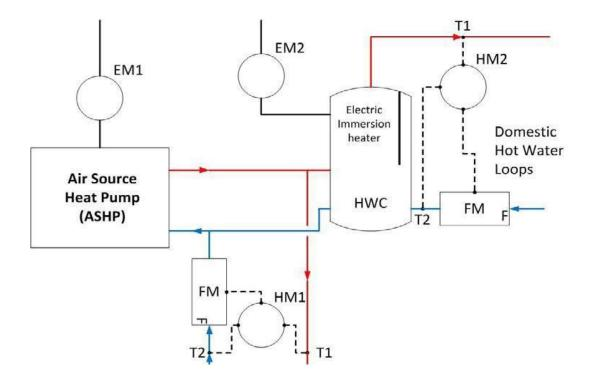
NOTE: One heat meter cannot be installed at the point that the pipes exit the ASHP due to physical constraints therefore must be installed as shown. One electricity meter is required to measure the input electricity required to run the heat pump compressor and any other electrical input plus given that the HWC cylinder has an additional electrical immersion heater it requires an additional electricity meter to record this electrical contribution to the metered heat output.
