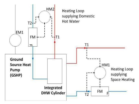
NOTE: Two heating loops exit the GSHP given that it contains an integrated Domestic Hot Water (DHW) cylinder (with no immersion heater). One loop feeds the DHW and the other the space heating.
