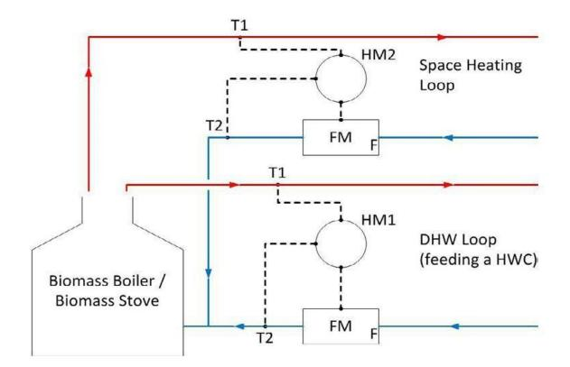
**Note**: This is a 3-pipe biomass installation using  $x^2$  flow pipes and  $x^1$  common return. It requires the installation of  $x^2$  heat meters.
