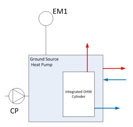
NOTE: Two heating loops exit the GSHP given that it contains an integrated DHW Cylinder (with no immersion heater). One loop feeds the DHW and the other the space heating.
