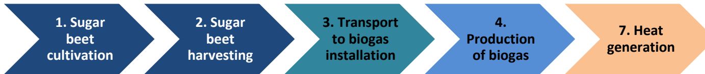
Figure 4: Example of a crop to heat generation fuel chain through the production of biogas: sugar beet (KEY: Dark blue: Cultivation and harvesting, Teal: Transport and distribution, Blue: Processing, Orange: Heat generation.)
